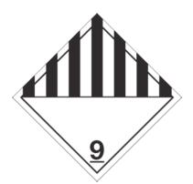
Use Class 9 Miscellaneous Dangerous Goods and UN Identification labels for transportation of lithium ion batteries which are assigned Class 9. Refer to relevant transportation documents.
